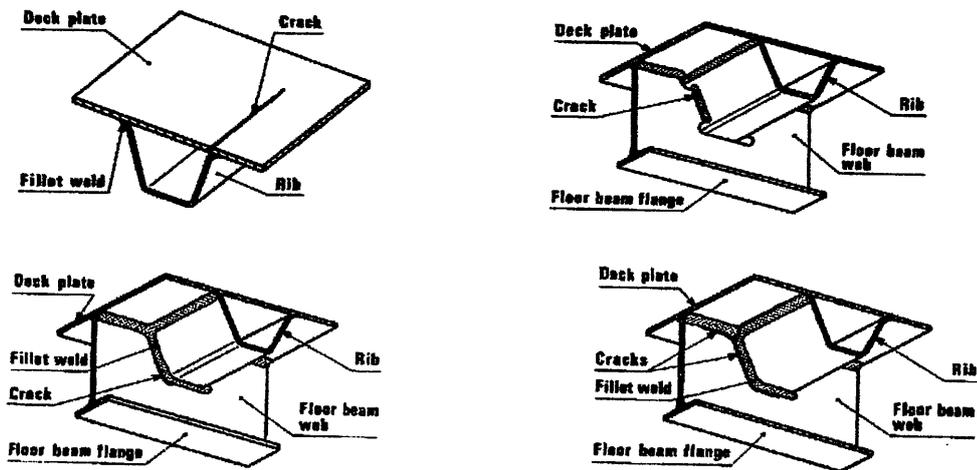
Gambar 2.13 Cracking in connections between cross girder and orthotropic steel plate
