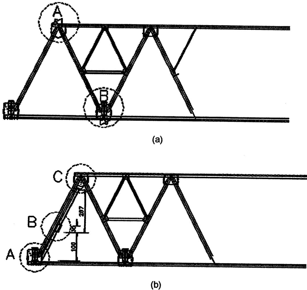
**Gambar 2.7** Replacing of tension chord and compression chord (A) placing external prestressed bar in replacing tension chord (B) placing jack supported by additional frame in replacing compression chord
