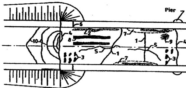
**Figure 2.2 Damage in paved roadway on concrete/composite bridges**
