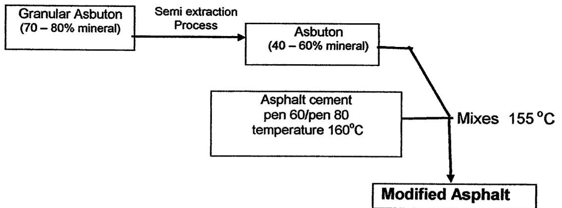
Figure 6.1 Process of modified asphalt cement by granular asbuton
