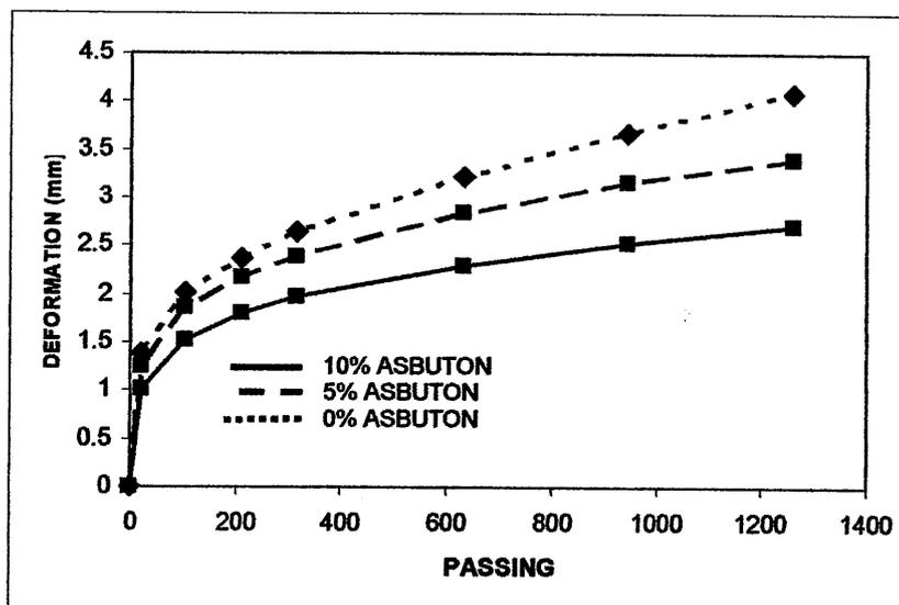
Figure 7.1 Graph showing the relationship deformation with passing
