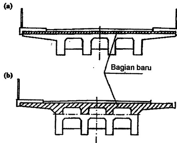
Figure 2.3 Strengthening by enlarging slab and beam sections
