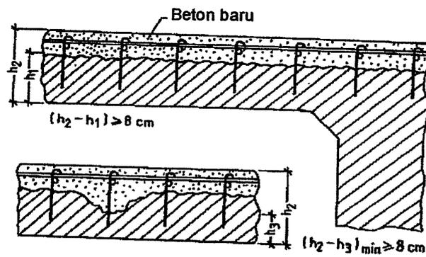
Gambar 2.4 Strengthening by enlarging deck slab section
