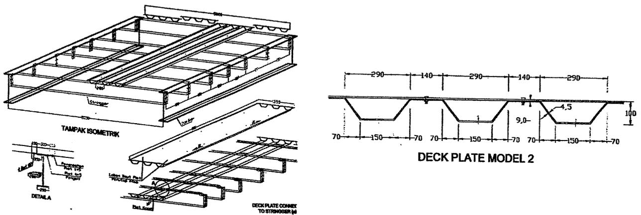
Gambar 2.12 Construction of orthotropic steel plate deck
