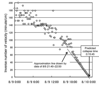
Application results of inverse number of velocity of extensometer displacement to forecast the time of slope failure
