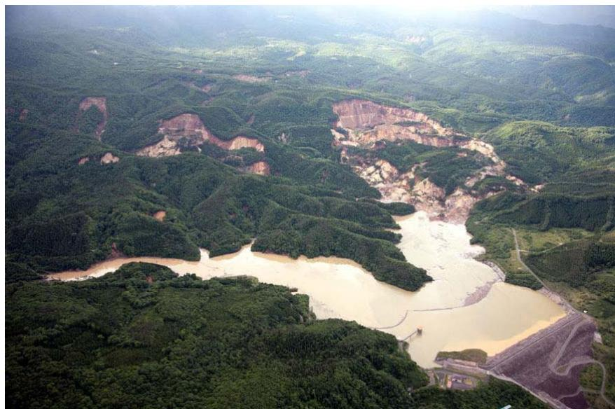
Downstream towards bottom, upstream towards top, of photo. Aratosawa Dam reservoir at center, with landslide occurring in its entire left upper tributary. The landslide has reached the reservoir. Multiple landslide areas apparent at left.
