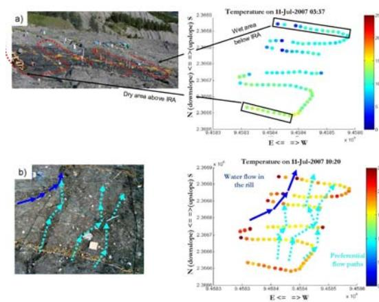
1 (a) Fibre Optic Cable installed within Infiltration Research Area (IRA) with temperature measurements and estimated preferential flow paths,
