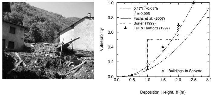
Empirical vulnerability function based on data from the 13 July 2008 mud-debris flow event in the village of Selvella (Valtellina study site): a function of deposition height.
