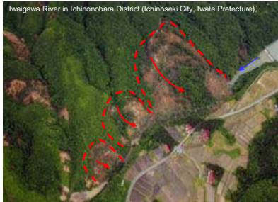
Natural Dam Blocking River Flow in Ichinonobara District
