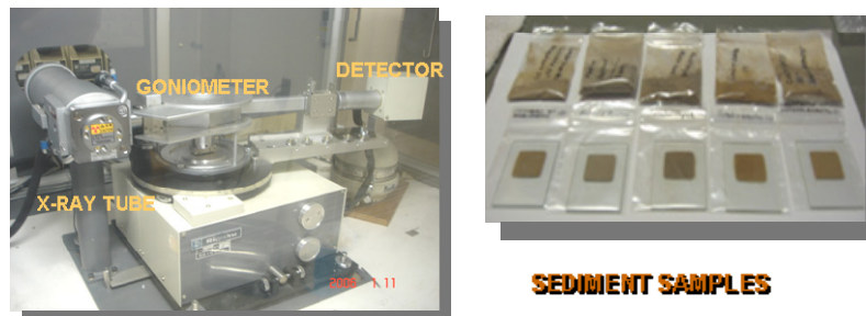
Figure 1. X-Ray Diffractometer and powdered sediment samples
