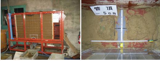
Soil Infiltration & Cave-in
