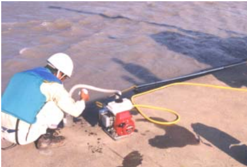
Suspended load being measured by the self-suction pump
