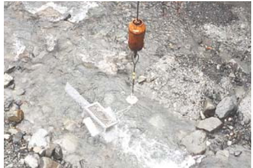
Observation of the amount of sediment discharge with the wire net sediment load catcher
