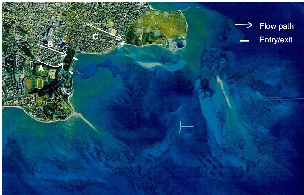
Figure 2.4 Freshwater drainage channel paths in Awase.
