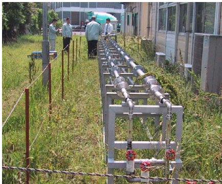
Set-up of steel water pipes coated with tar epoxy resin paint ( \phi 32 and 40mm) which were continuously supplied with treated water containing residual chlorine
