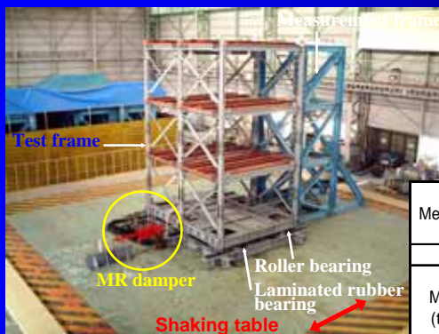
base-isolated test frame Parameters test frame
