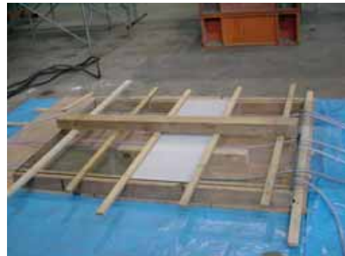
Photo 1 Filling test of non-shrinkage mortar
