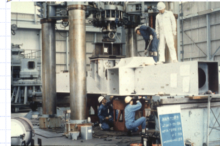
Real scale floor beam of the Seto Bridge
