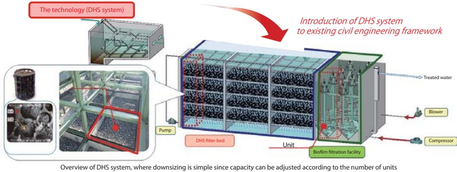
Overview of DHS system, where downsizing is simple since capacity can be adjusted according to the number of units
