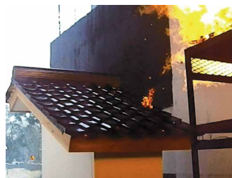
Photo 1 Test of fire ignition by sparks
