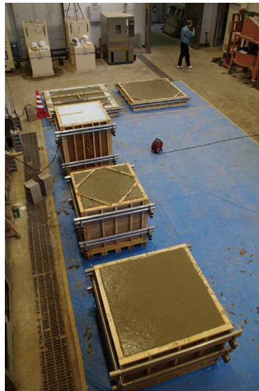
Photo 1. Full size specimens being prepared
