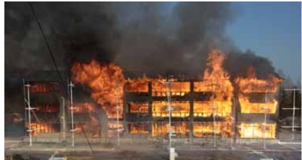
View 34 minutes after ignition, when the fire had spread to the entire building.
