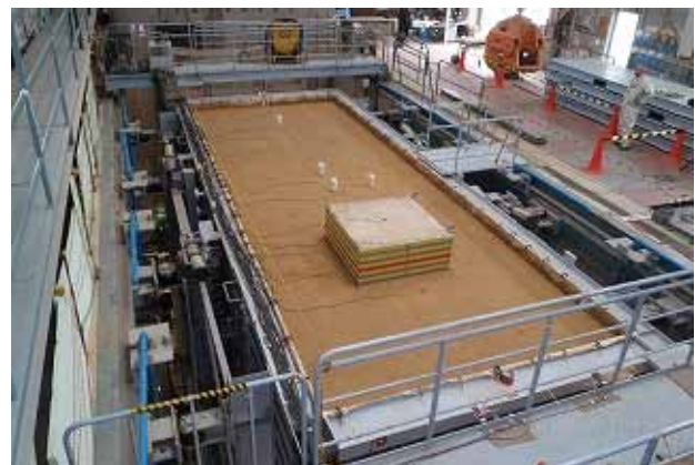
Photo: Large scaled specimen of sand ground for the seismic liquefaction test
