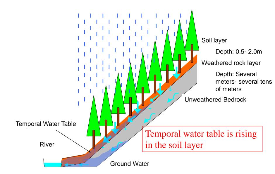
How does a landslide occur when the situation is like this?
