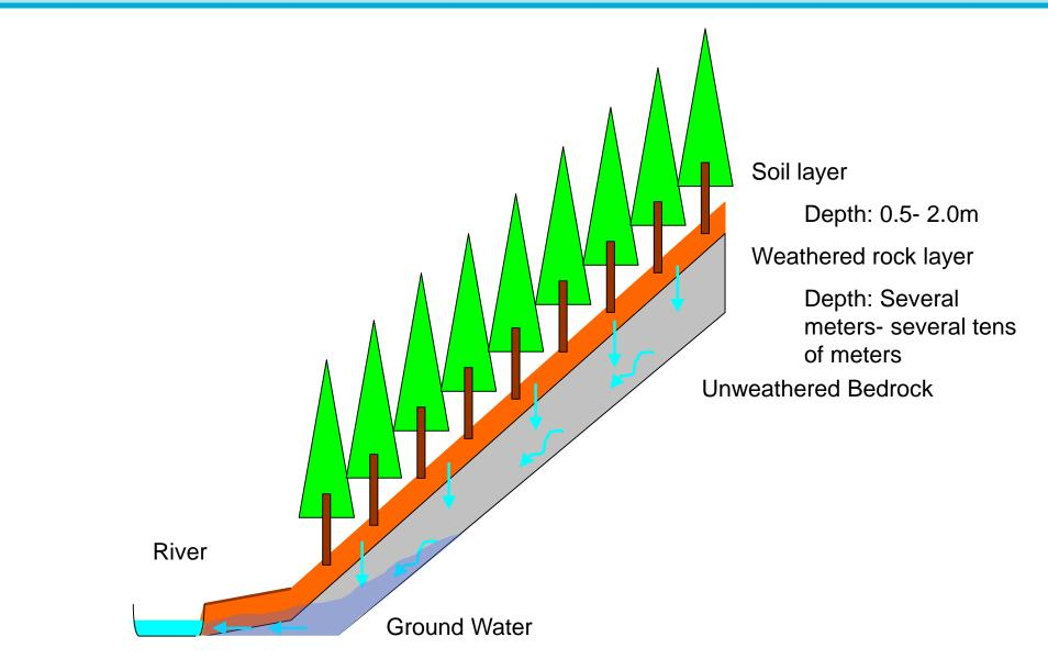
How does water flow when it rains?
