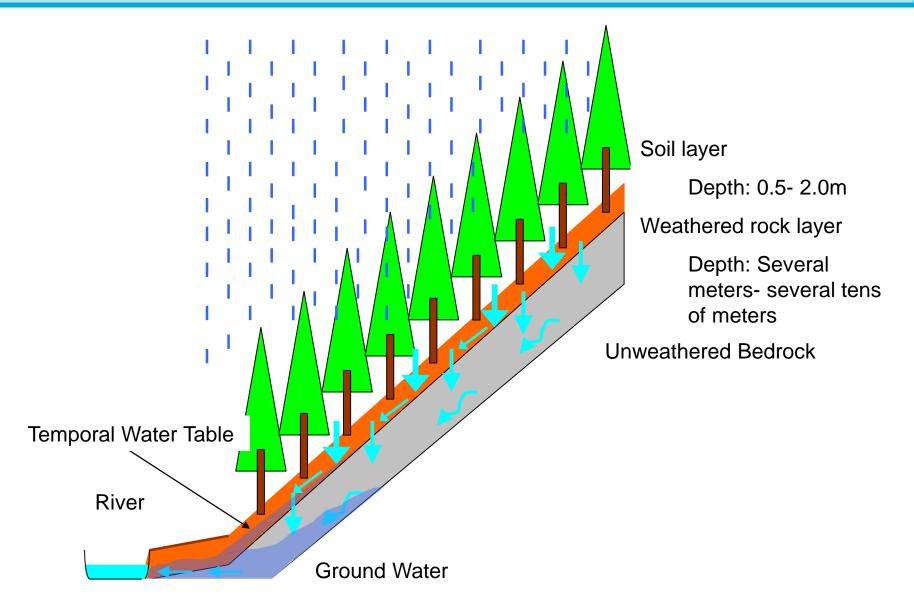
If a weathered rock layer is impermeable...
