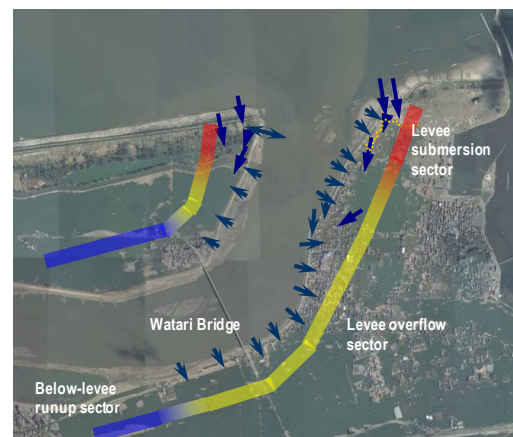
Photo 3.2.2.1(d) Status of Tsunami Runup into the Abukuma River
