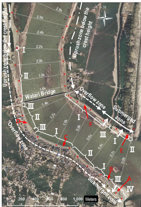
Photo 3.3.3.1 Relations between high water level of the tsunami and height of levees and the extent of damage
