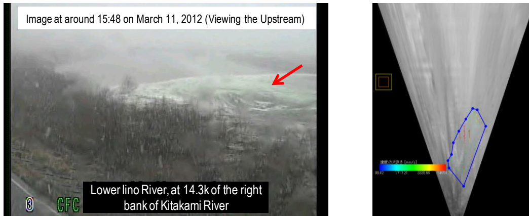
(a) Image extracted from the CCTV image (arrow shows the tsunami wavefront) (b) Result of PIV analysis of a planar projection of the image on the left
