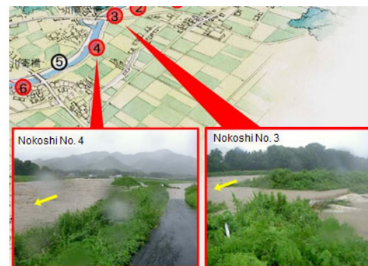
Fig. 2: Nokoshi, letting overflow for damage reduction
