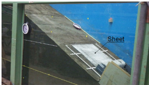
Photo 3: Pull-out resistance measurement experiment
