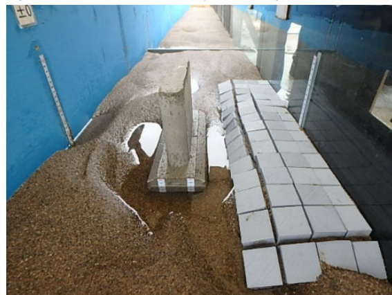
Photo. Experiment on scouring around streambed protection
