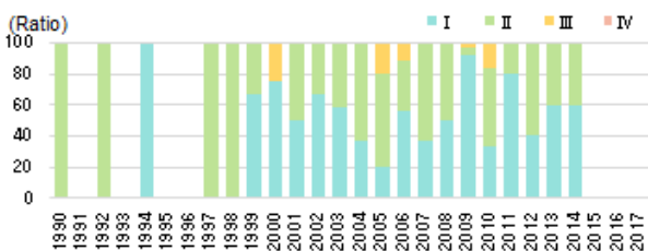
Fig. 9: Percentage of judgment categories by construction year (Precast culvert, since 1990)
