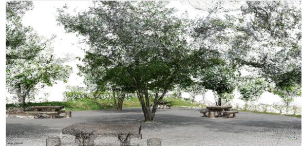
Figure 4: Point cloud data created from photos taken by digital cameras
