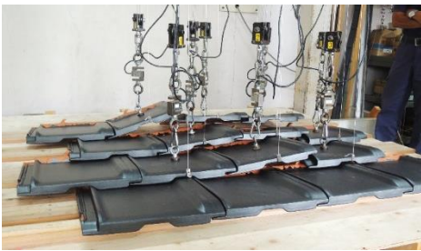
Photo 2: Tension loading test on the upper part of a tile roof
