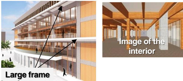
A government building with a wooden structure installed within a large frame double-layer RC structure.
