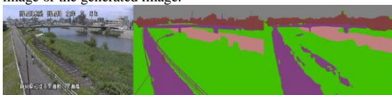
Fig. 4 CCTV camera image in a normal state (left), correct answer annotation image (middle), generated annotation image (right)
