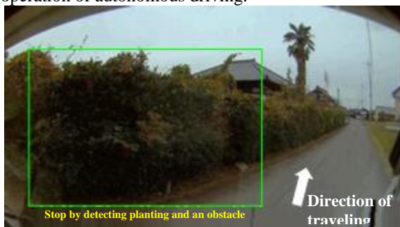
Fig. 4 Detection of planting as an obstacle
