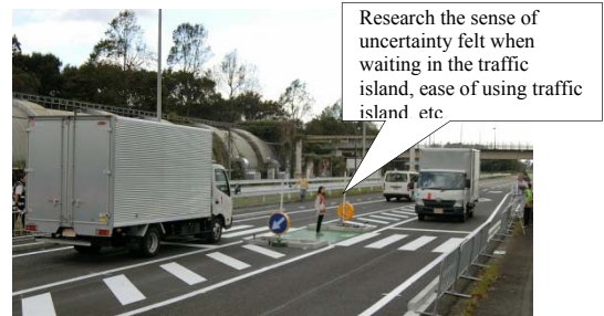
Fig. 2: Traffic experiment with a temporarily built two-stage crossing facility
