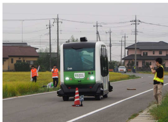
Photo: Automatic driving experiment at Roadside Station Nishikata
