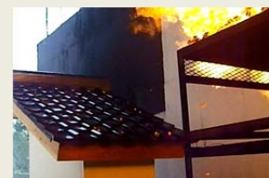
Experiment of scattering fire using tiled roofs
