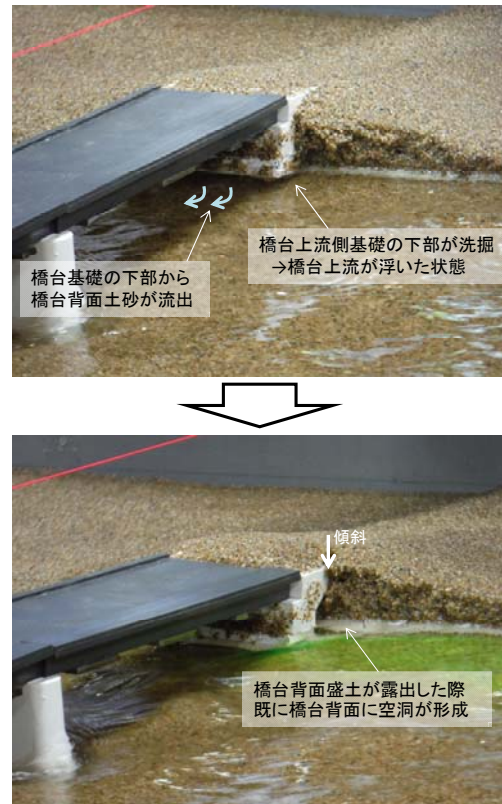
Fig. 4 Cavitation of the abutment back by sucking from under the abutment
