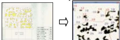
Fig. 1 Example of showing, in the form of texture data, sections of exterior walls where wall exfoliation hazards may exist as described in exterior wall investigation reports
