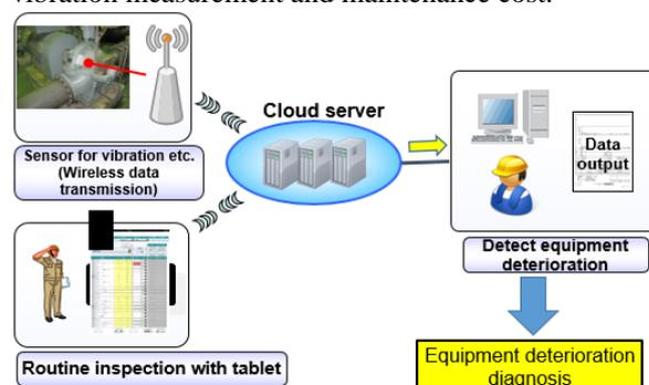
**Figure 2: Sensor continuous monitoring and cloud server consolidation technique**
