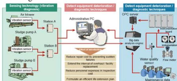
**Figure 1: Sensing technology and big data analysis technology**
