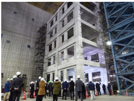
Photo 1. Full-scale static loading test on five-storied building
