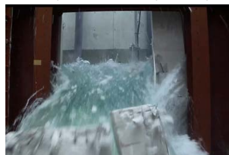
Photo 2. Hydraulics model test in which exterior wall claddings are destroyed by water pressure
