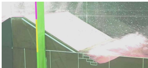
Photo: Experiment with a model (Case (8)) Anchoring works + Stacked blocks
