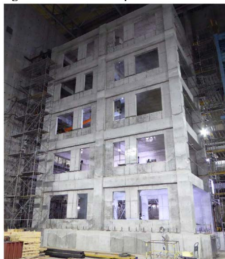
Photo 1. A test using an actual-scale five-layer reinforced concrete structure to propose structures that will not require repairing columns and beams after a massive earthquake
