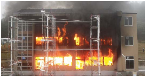
Photo 2. Actual-scale fire experiment to verify the adequacy of specifications to set standards for three-story wooden school buildings
