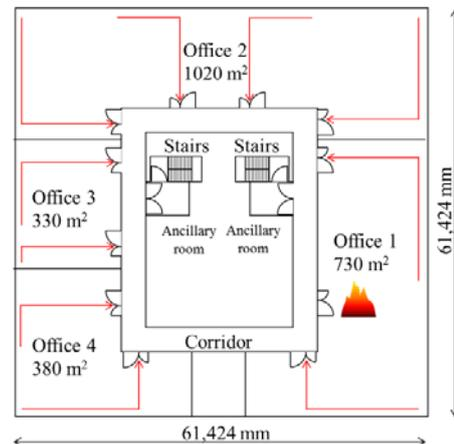
Fig.-3 Floor plan of offices used for calculation of risks
