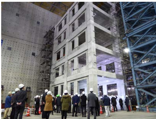
Photo 1. Damage test using an actual-scale five-story building
