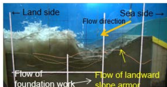
Photo: Experiment of break from the landward slope foundation work
