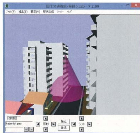
Figure. An example of a viewer that visualizes the risk of falling outer walls
