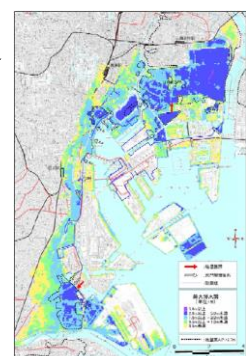
Fig.-2 Example of storm surge inundation calculation
