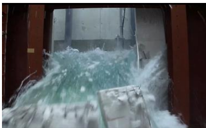
Photo 1: Hydraulic test on external walls
