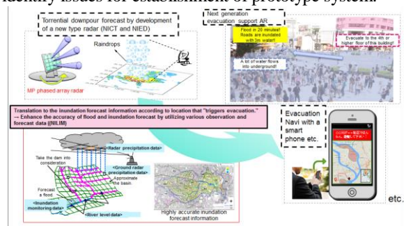
Figure 1. Concept of Collaboration in Technical Development for the Observation, Analysis, and Forecast of Flood Disasters
