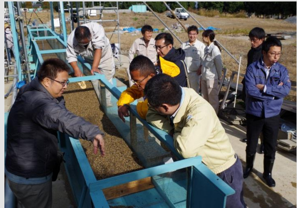
Photo 1: Exercise with Flume Experiment concerning Landslide Dam Breach and Countermeasures
