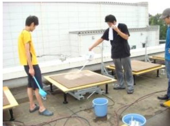
Figure 1: Watering to experimental sample of water retentive building material
