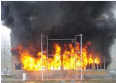
Photo 1: Fire spread to the 2nd floor
