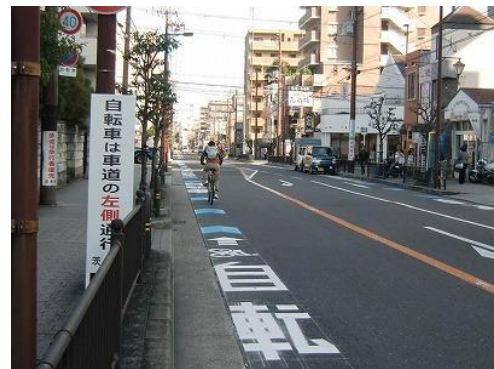
Photo. Example of a Mixed Traffic Lane
