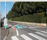
In the first section, a narrow road shared by automobiles and pedestrians, the roadside strips were widen and colored in order to ensure space where pedestrians can walk safely.
