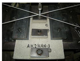
Photo 1 Direct tensile test
