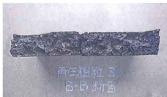
Photo 1 Specimen of asphalt concrete with recycled aggregate after immersed wheel tracking test
