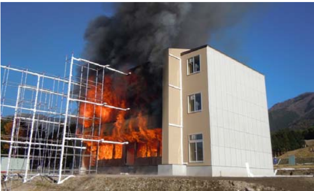
Photo: The spread of fire to the second floor at the time of 137 minutes after setting fire
