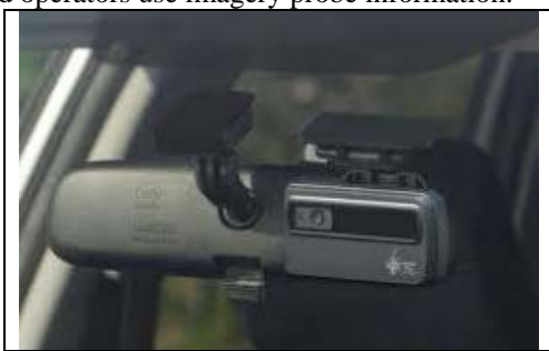
Photo 1. Example of an In-vehicle Camera Installed on a Rear-view Mirror
