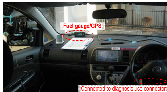
Photo 1. View of Installation of Fuel Gauge in an Automobile
