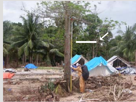
Photo 1. Measuring trace height (white line shows trace height)
